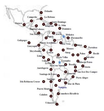
**Figure 1:** Ground network topology **Source:** GMV PT report No. 2100, Technical analysis of the SACCSA SBAS solution
